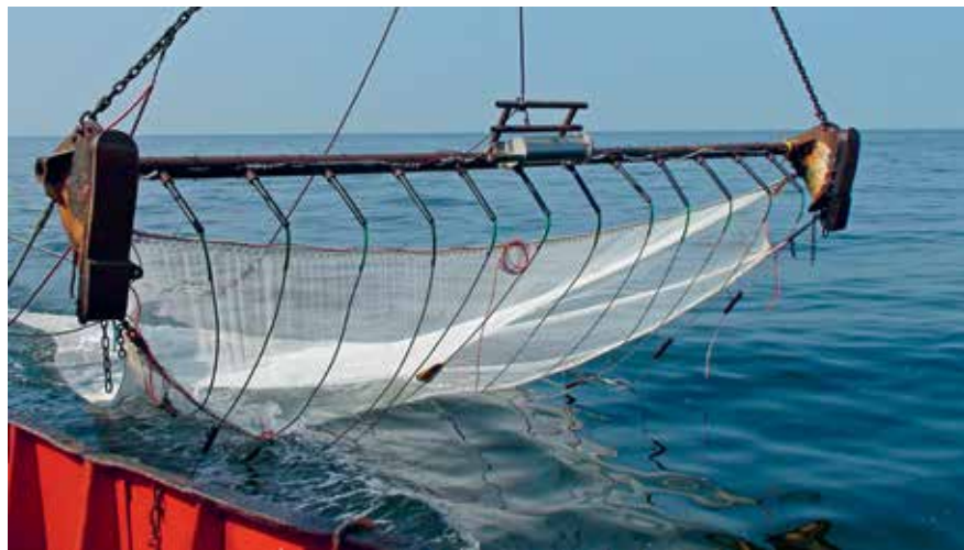
Figure 8: The HOVERCRAN with 8 m beams, trawl shoes and 12 electrodes of 3 m length each. Source: Soetaert et al. 2013.
